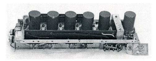
Figure 5: Receiver Unit Type 153 (the Pye 45MHz IF strip).
