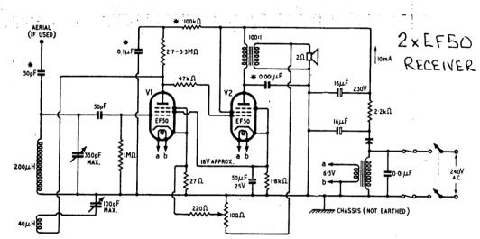
Circuit diagram of the receiver. Resistors can be  $\frac{1}{2}$ W and capacitors 350V d.c. working. The 0·01- $\mu$ F capacitor across the mains input must be capable of continuous operation at 250V a.c. Components marked thus \* may be omitted for 'local' reception. The cathode resistor for  $V_2$  must be adjusted to fix the h.t. current at 10 mA.
