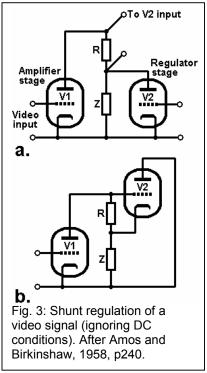
the extra loadcurrent demand. It is obvious that V2 is in parallel with the load and maintains or regulates the signal against a falling load impedance at increasing frequency. From this principle it is a short step to the SRPP in fig. 3b.
