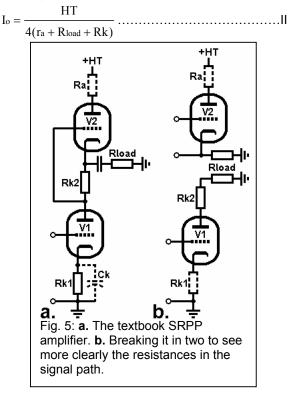
How can we force the quiescent current to equal this ideal value, for a given load impedance? There must be an optimum value of bias resistance Rk which will achieve this. This value is easily found by equating I and II (and remembering to add the extra resistor Ra). Thus we find the optimum value for the bias resistors:
