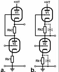
Fig. 4: **a.** With an infinite load the circuit is not an SRPP at all, but an actively loaded triode. **b.** By moving the output to the anode of V1 we obtain the *half-µ stage*. Bypassing both resistors reduces the output impedance, but distortion will be greater.
