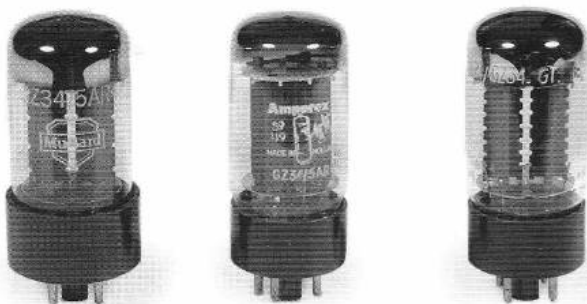
Mullard GZ34 (wide base), Amperex GZ34, Sylvania GZ34
