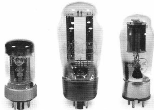
Metal-Based Mullard GZ34 (1950s), Genalex U52 (1960), and Russian (Svetlana) 5U4C (1950s)
