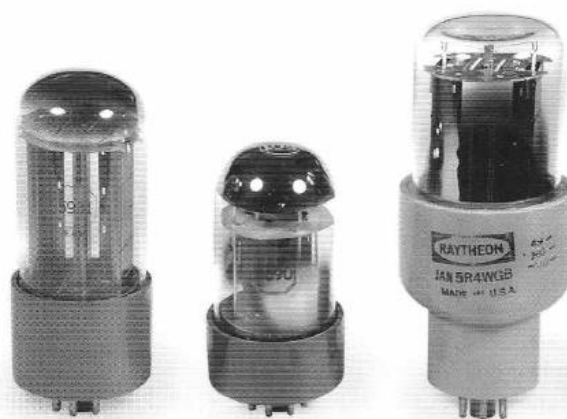
Military Octal Rectifier Types: Sylvania 5931, RCA 5690, Raytheon 5R4WGB
